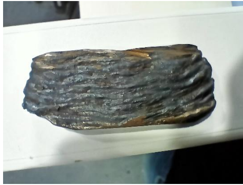
3-D printed metal part – through Yaskawa Arc Welding Robot
