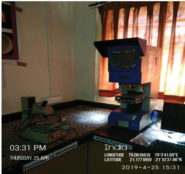
Toolmaker's Microscope and Profile Projector for measurements of thread, major-minor diameters.
