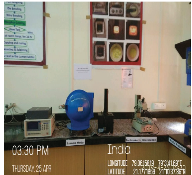
Lumen Meter for measuring LED characteristics
