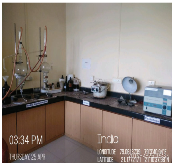
Double Distillation Unit, Oil Bath & High Speed centrifuge
