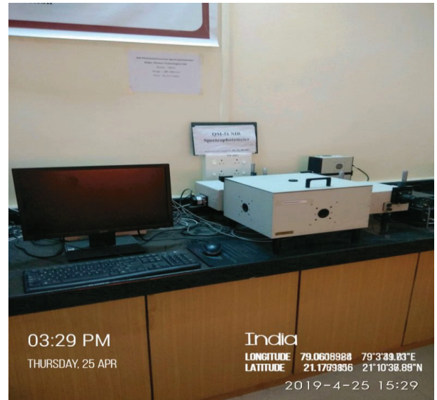
Near Infrared Spectrophotometer Quantum Master QM-51 Photon Technologies USA for measurement of fluorescence in NIR region
