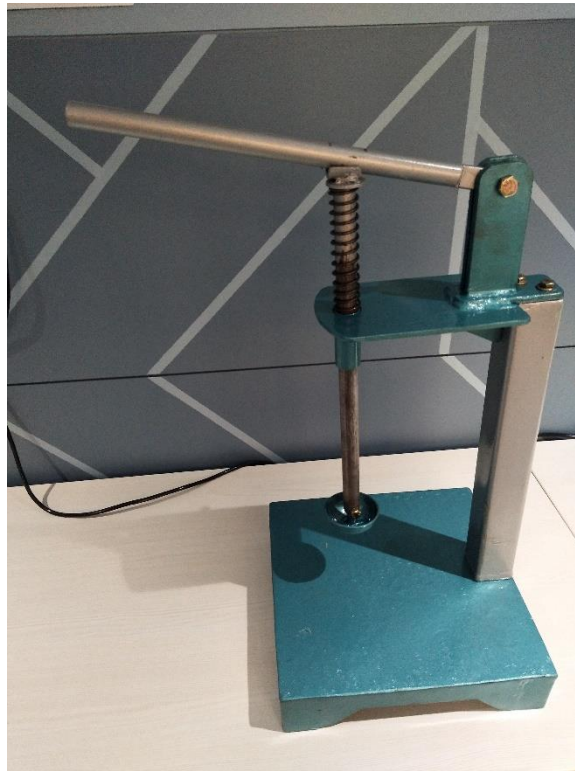
Portable Hand press machine, designed and fabricated for SGVAK
