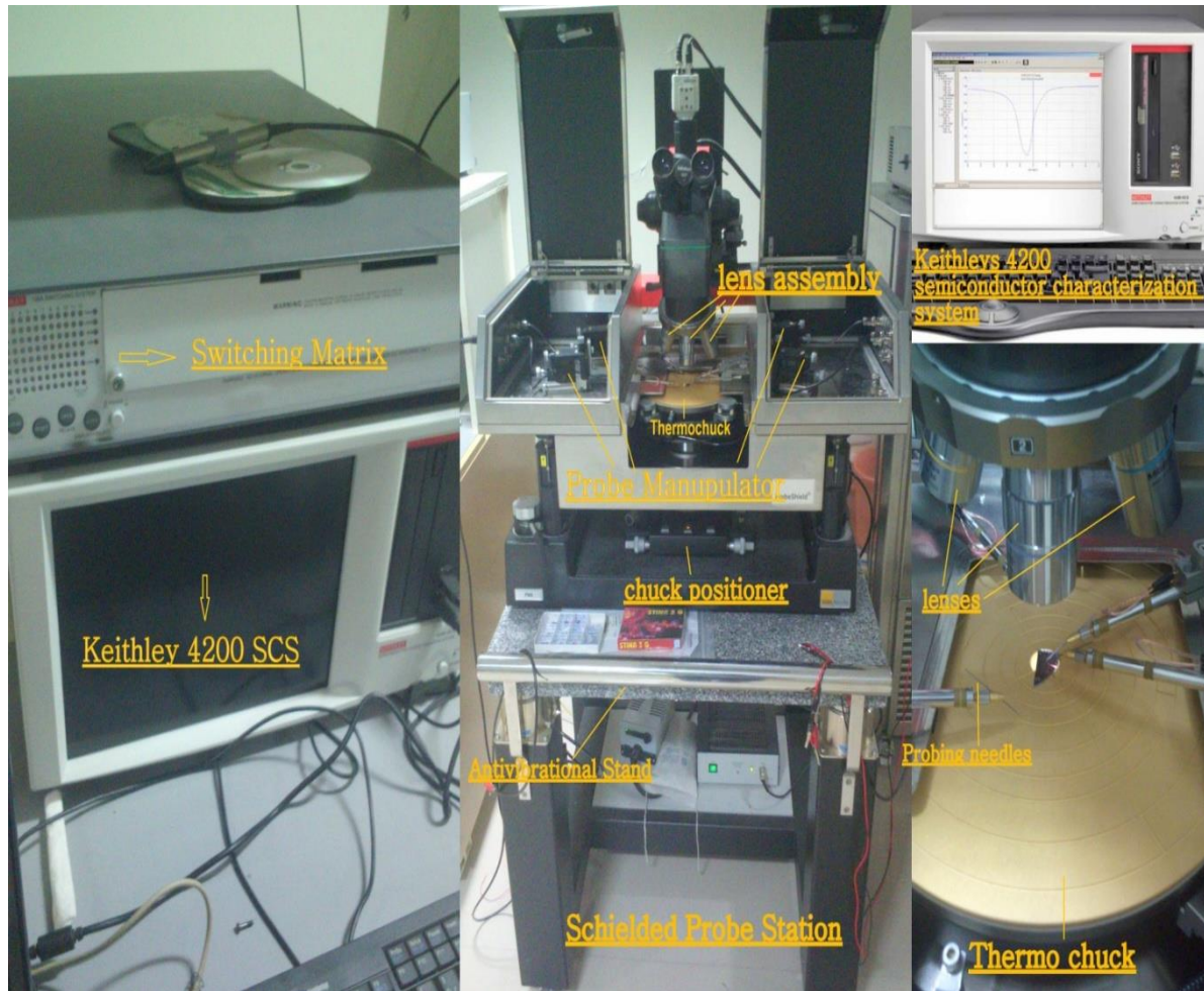
Fig. 16. Electrical characterization setup
